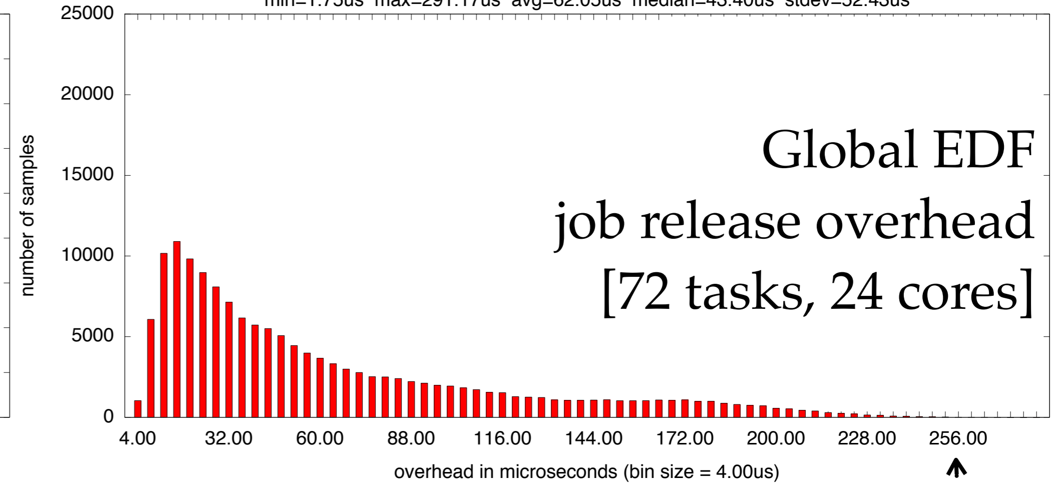
G-EDF: measured job release overhead for 3 tasks per processor (host=ludwig) min=1.75us max=291.17us avg=62.05us median=43.40us stdev=52.43us
